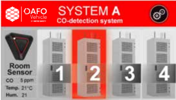
Image E - The display shows the affected cabinet in red
