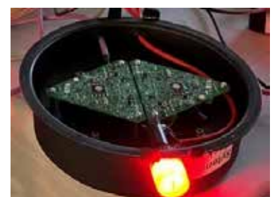
Image D – a top box containing sensors, fan and beacon
